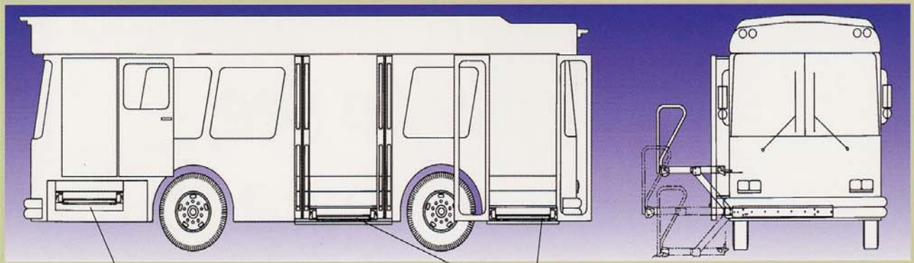
Locate unit beneath dedicated door or in modified luggage compartment. This application combined with track seating maximizes seating capacity.
